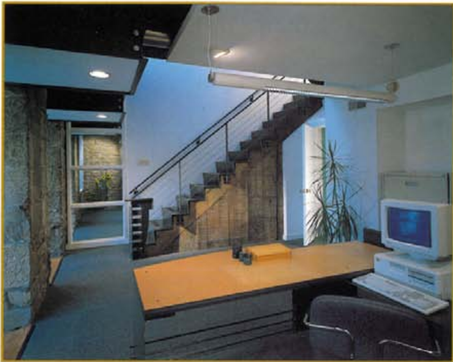
A casual seating and reception area is located just inside the building's entrance. The architect tore out the original staircase connecting the first and second floors, and designed a modern version reaching to the third story. Steel beams and cables were arc-welded in place, bringing inside some of the materials introduced in the vestibule.
